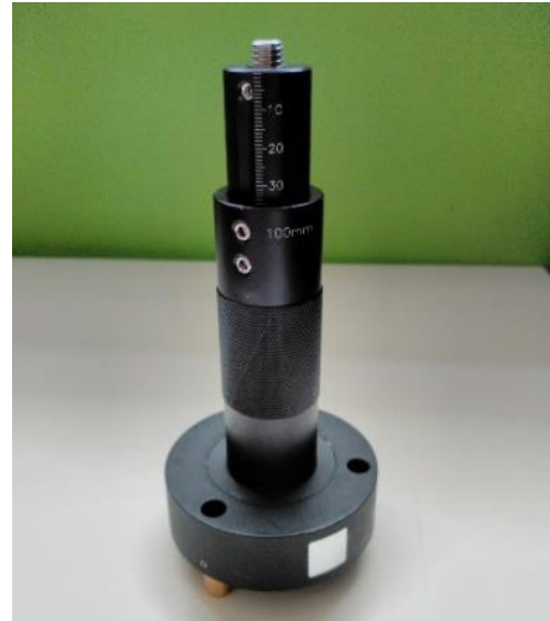
Img. 02.03. Adaptor rod and Tribrach setting to achieve the right position for works with Leica P40 laser scanner.
