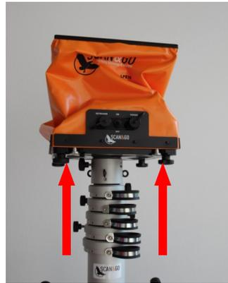
Tighten the 4 locking knobs
