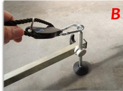
Connect the wind bracing ropes to the stabilizer feet like
