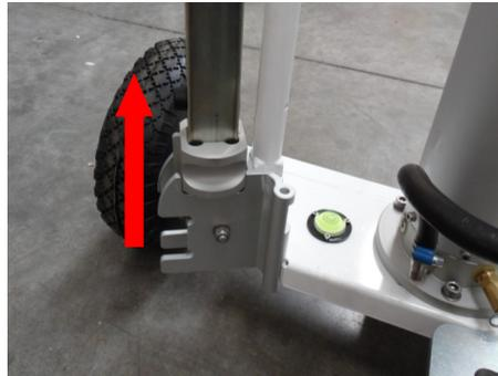
Extend outwards the skates and rotate the stabilizers until the skates click into place
