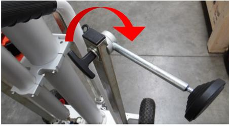
Loosen and rotate the adjustable foot bases 90° outwards
