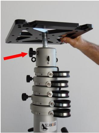
Place the plate on the top-head of the structure and tighten the locking screw
