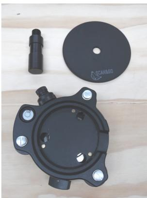
Insert the pivot with the 5/8" male with the round plate thread to the Trilock
