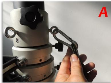
Connect the wind bracing ropes to the top- head of the structure
