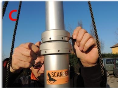
Close the mechanical lock of the first extension and open the one of the second one
