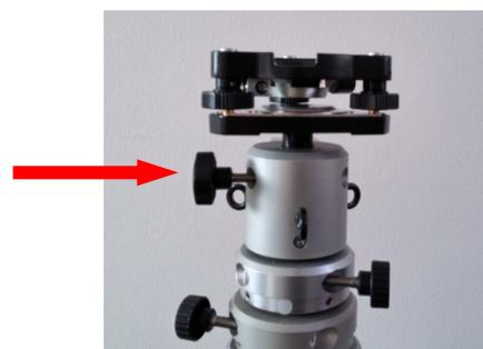
Insert it into the top-head of the structure by tightening the locking screw
