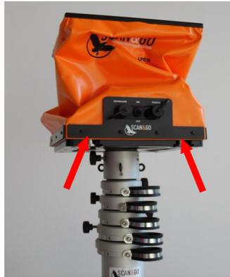
Place the LP16R using two pins
