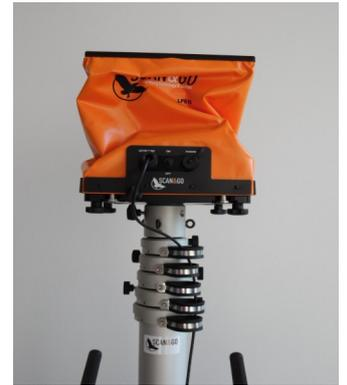
Insert the connecting cable inside the cables glands
