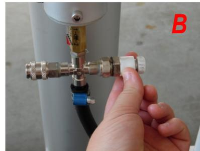
Open the air safety valve for the descend of the first extension.
