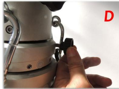
Fully open the mechanical lock of the first extension
