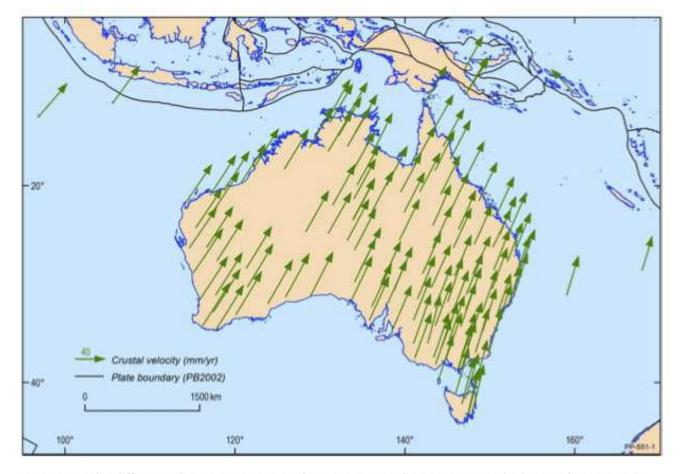
Figure 3.1: The difference between GDA94 and GDA2020 coordinates is primarily due to plate tectonic motion.
