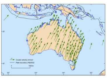
Figure 3.1: The difference between GDA94 and GDA2020 coordinates is primarily due to plate tectonic motion.
