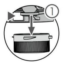
Align the white dot on the AA450 Skyport interface with the red dot on the M300 interface and embed it in the installation location.
