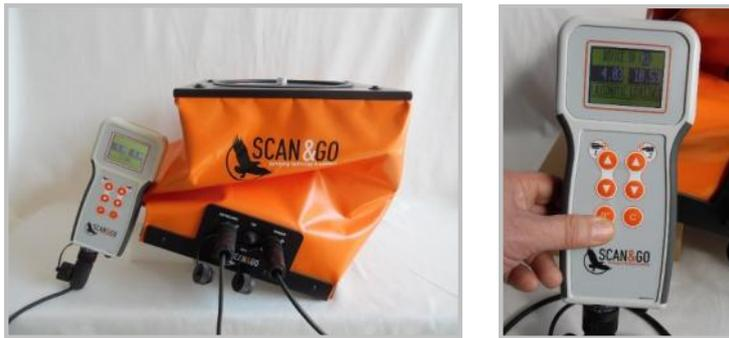
Simply press a button, the system proceeds automatically reaching the horizontal position on both axes.
