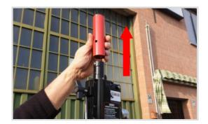
Keeping the safety lock pressed, insert the terminal into the extension and tighten the stop with the Allen key
