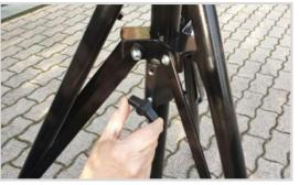
**NOTE** Before moving the pole upwards, loosen the knobs.
