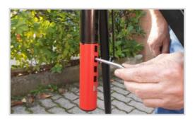
With the crank lift the pole up to the starting point of the red safety terminal and lock with the side knob
