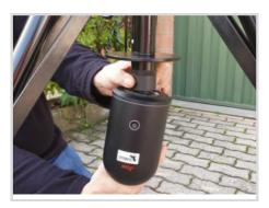
Using the supplied Allen key, unlock the safety terminal
