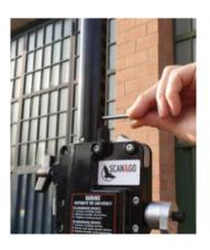
Hold down the safety lever and rotate the crank to lower the scanner
