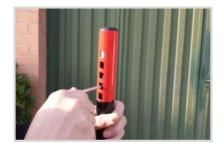
While holding down the safety catch, insert the extension and lock with the Allen key
