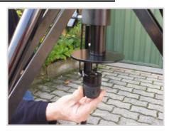
Screw the adapter into the 5/8 "thread terminal and insert the scanner
