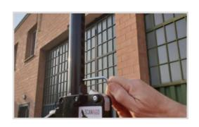
Insert and lock the safety terminal in the lower part
