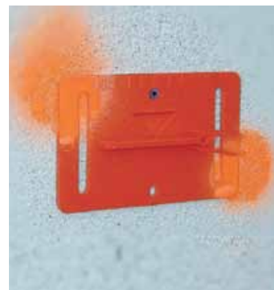
RS21r glued, fastened and sprayed on with colour - manipulation is thus prevented.
