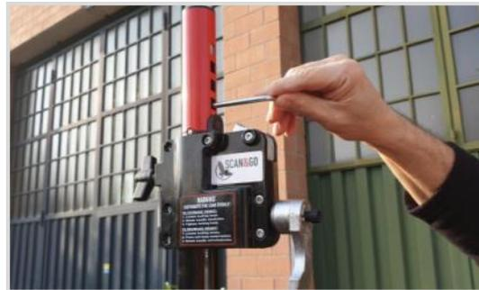
Holding down the safety catch, slide the terminal upwards
