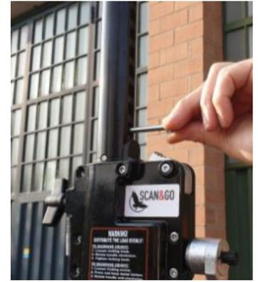
Hold down the safety lever and rotate the crank to lower the scanner
