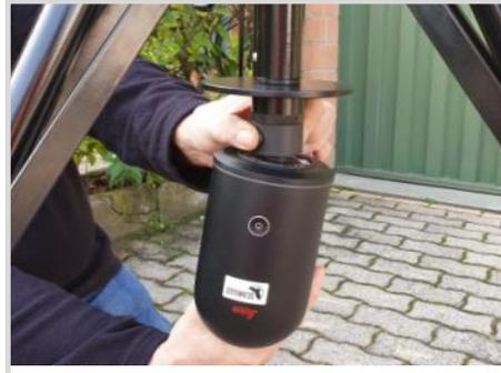
Using the supplied Allen key, unlock the safety terminal
