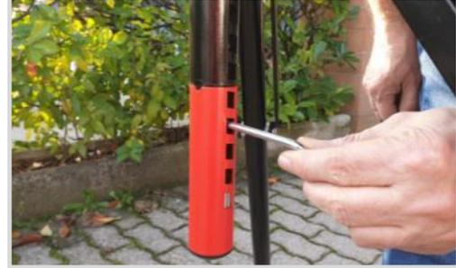
With the crank lift the pole up to the starting point of the red safety terminal and lock with the side knob
