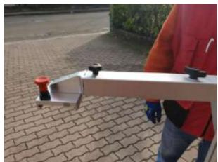
Lower the ballast support and place the ballast bag, ATTENTION, the support should never touch the ground.
