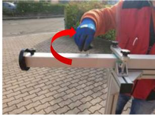
To use the head with safety adapter for vertical scanning (head up or head down) replace the head with 5/8" attachment
