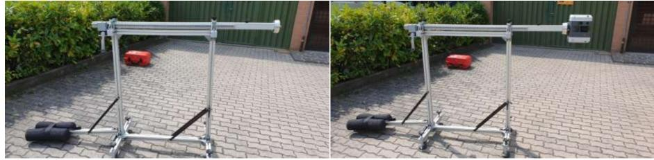
Insert the extension and screw the stop bolt
