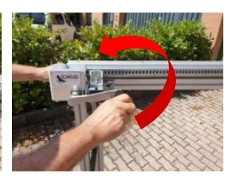
Insert the two upper runners without tightening the locking knobs too much as the extension must be able to slide
