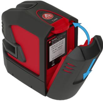
Insert the battery-pack by pressing it down and then tilting it towards the housing as shown until it snaps in.
