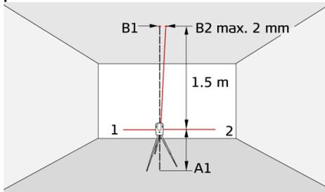
Place the lock switch in the "Unlocked" position (see [Levelling lock](#)). Set up the laser on its tripod to wall mount bracket near point A1 at a minimum distance of 1.5 m from point B1. The horizontal laser is aligned in direction 1. Mark the laser points A1 and B1 with a pin.
