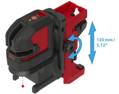
Turn the adjustment knob of UAL130 to fine adjust the horizontal line to the desired reference level.
