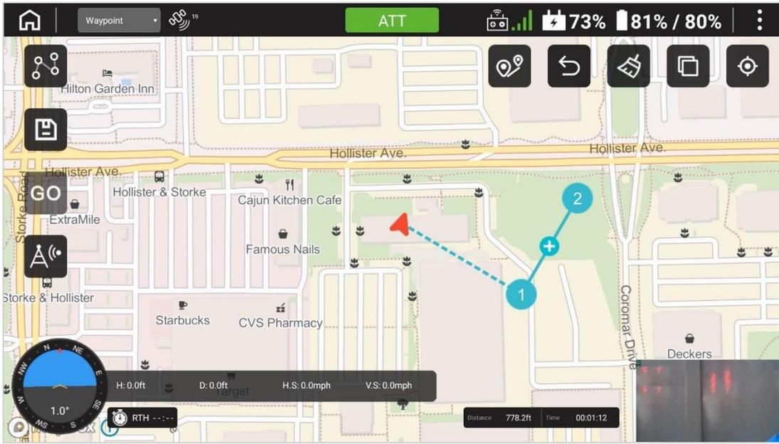
FIGURE 8.H DRAWING THE FIRST TWO WAYPOINTS
