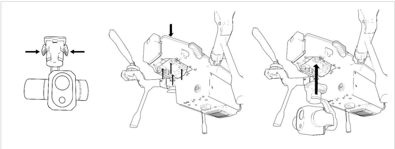
FIGURE 6.E CONNECT THE PAYLOAD USING THE QUICK RELEASE, RAILS, AND CONNECTOR
