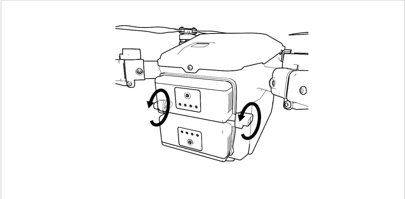
FIGURE 6.D LOCKING THE BATTERIES IN THE AIRCRAFT
