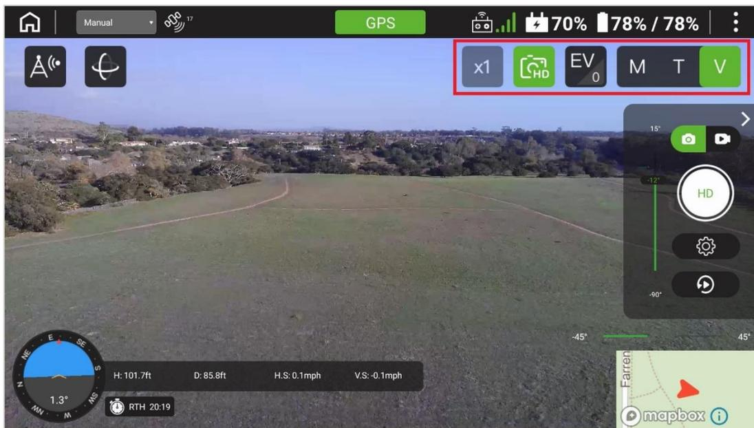
FIGURE 7.O VISIBLE CAMERA QUICK-ACCESS FEATURES
