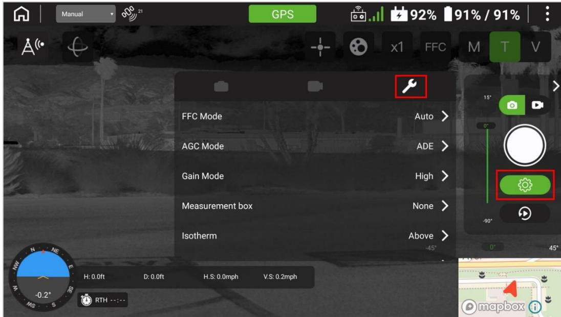
FIGURE 7.Y RADIOMETRIC ADJUSTMENTS FOR THERMAL CAMERA
