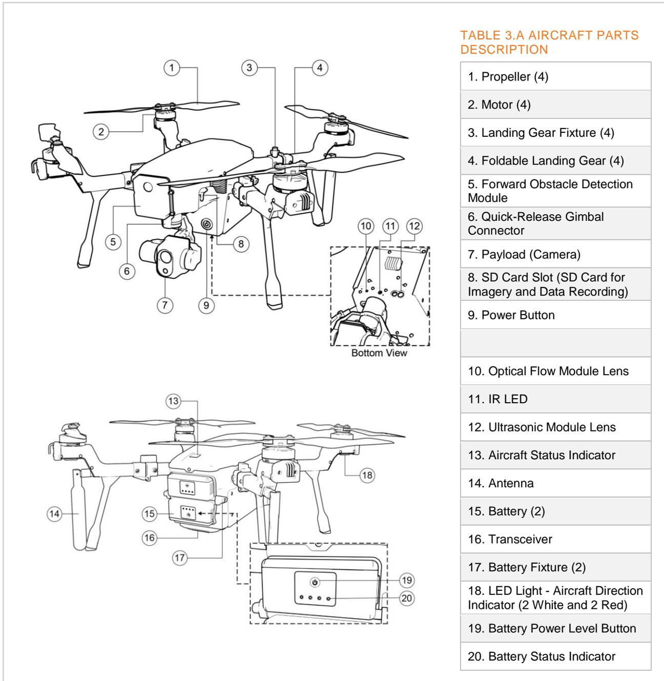
FIGURE 3.A SIRAS AIRCRAFT FRONT AND REAR VIEW
