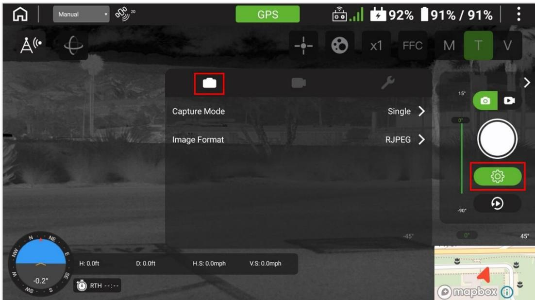
FIGURE 7.W CAPTURE MODE AND IMAGE FORMAT SETTINGS FOR THERMAL CAMERA
