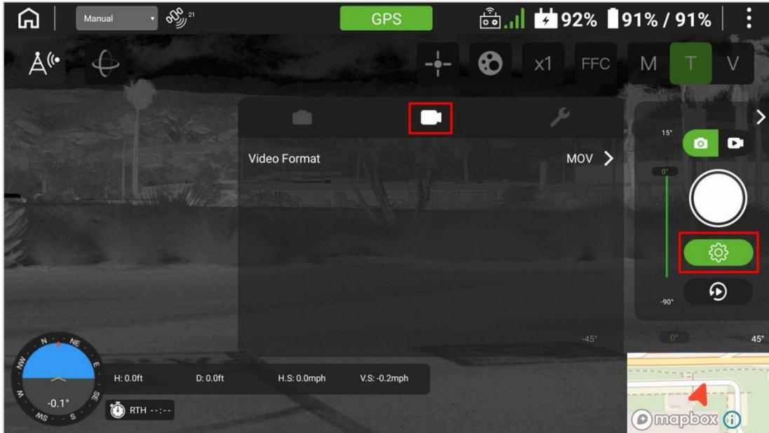
FIGURE 7.X VIDEO FORMAT SETTINGS FOR THERMAL CAMERA
