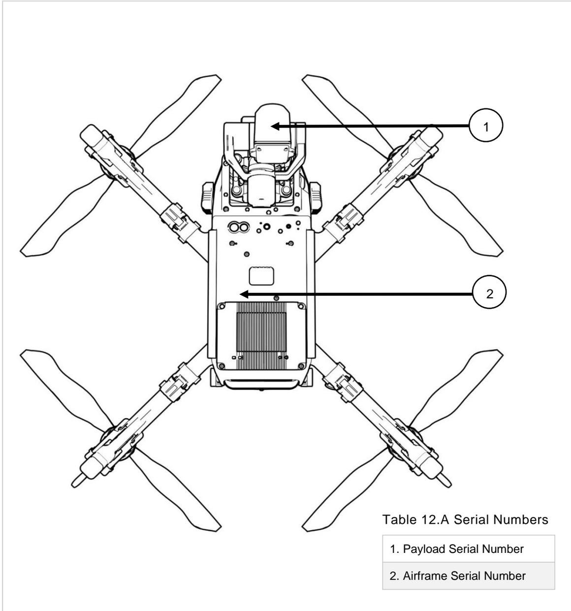
FIGURE 12.A PAYLOAD AND AIRFRAME SERIAL NUMBER LOCATIONS
