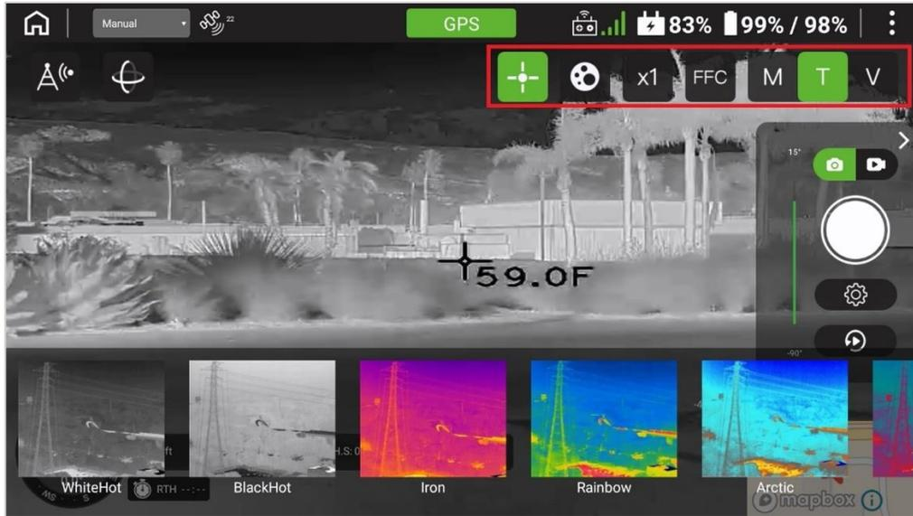
FIGURE 7.Q THERMAL CAMERA QUICK-ACCESS FEATURES
