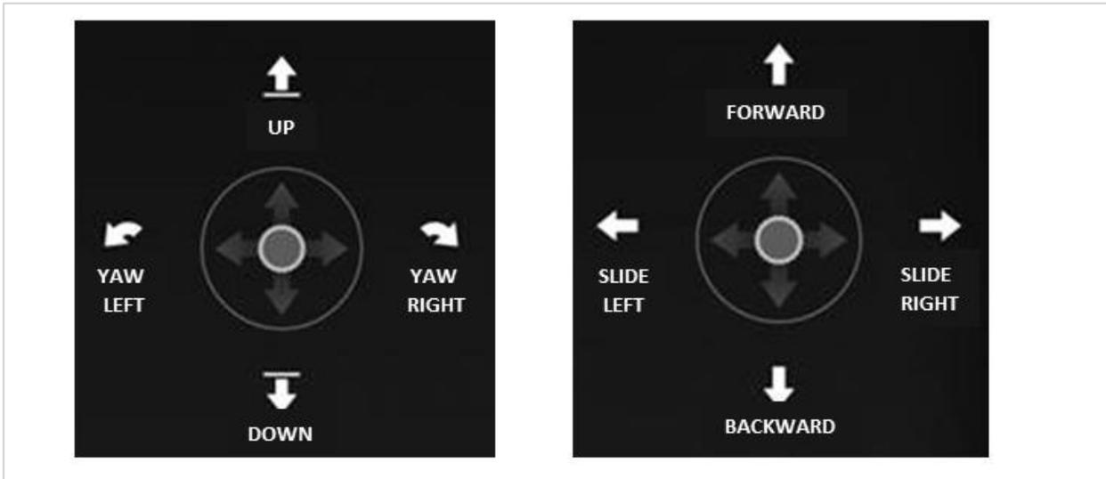
FIGURE 8.F JOYSTICK CONTROLS (LEFT AND RIGHT, IN MODE 2)
