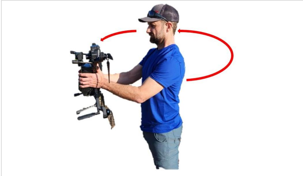
FIGURE 8.C COMPASS CALIBRATION STEP 3: HORIZONTAL ROTATION, NOSE-UP
