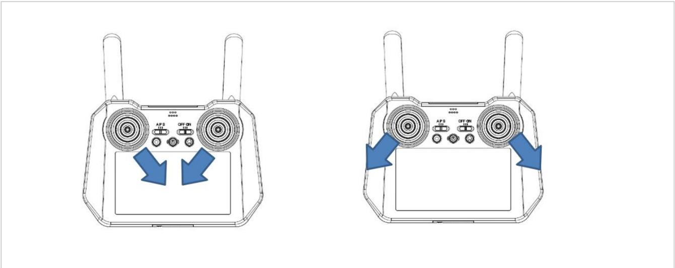
FIGURE 8.E TURNING MOTORS ON (LEFT) AND OFF (RIGHT)
