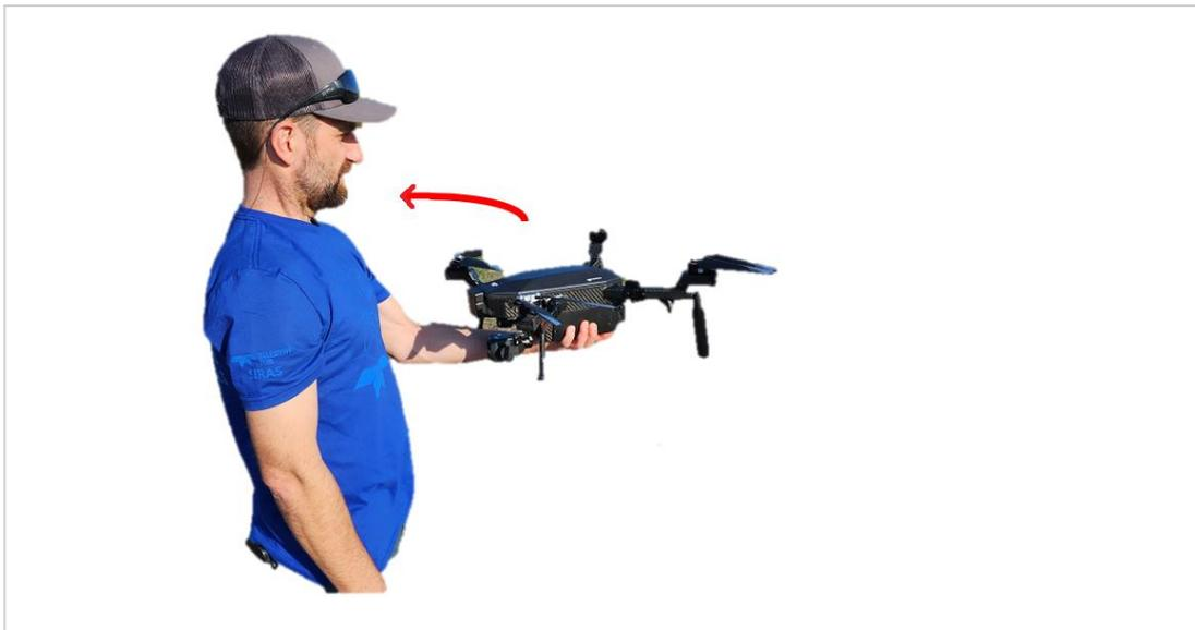
FIGURE 8.B COMPASS CALIBRATION STEP 2: HORIZONTAL ROTATION, LEVEL
