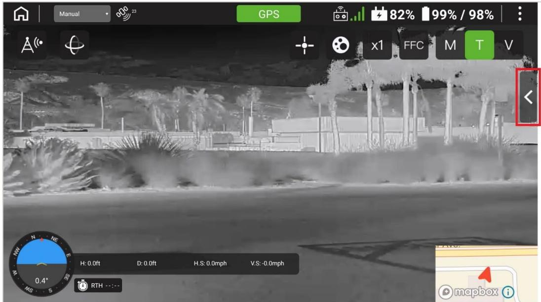
FIGURE 7.U BUTTON TO EXPOSE HIDDEN SHUTTER CONTROLS
