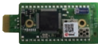
vLoc3 Series Bluetooth Module
