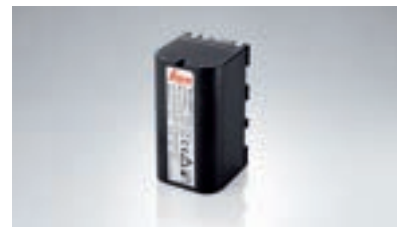
GEB221, Li-Ion battery High output battery for all TS02/06/09/11/12/15/16, GS10 GNSS receiver and Piper 100/200, 7.4 V / 4.4 Ah. Order No: 733270
