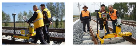
A design tool was used to reconstruct the best-fit track parameters based on as-built track position. The deviations from the reconstructed track design can be used as correction values, which can then be transferred to the tamping machines.
