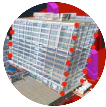
Virtual Building with Construction Layout Points
