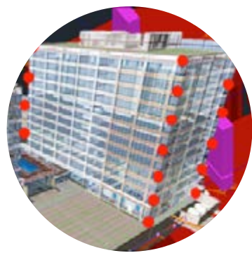
Virtual Building with Construction Layout Points
